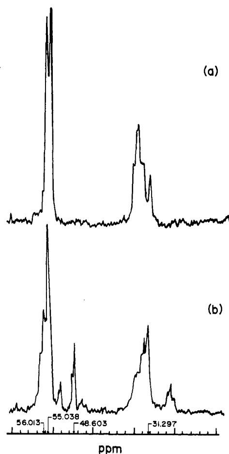
Figure 2. 13 C NMR spectra: (a) reference sodium poly(vinylsulfonate) (PVS-2); (b) matrix polymerized sodium poly(vinylsulfonate) (PVS-1).
